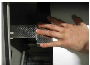
While the paper feeds into the processor, check with your hand if the paper stays straight.
