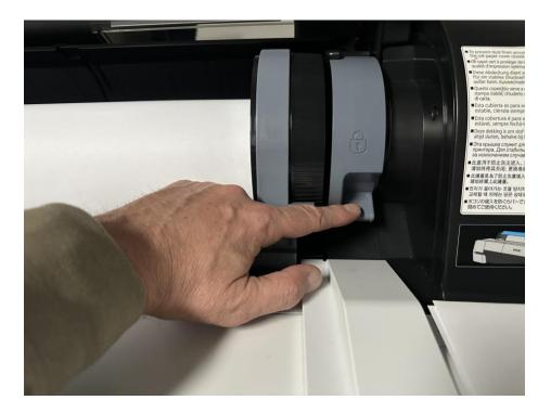
Close the roll paper cover. Always keep the cover closed unless loading or unloading media.
