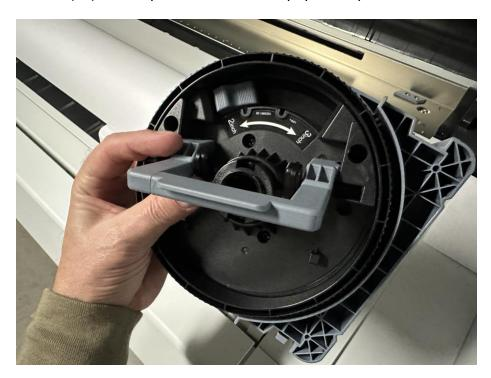
Push adapters into the paper core at both ends of the roll and push down the adapter lock levers flat against the adapters.
