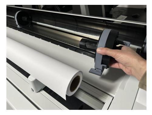
Make adjustments for the desired roll diameter (Bond 44" has 2" core, all the other papers have 3" core) by sliding the size lever to the side that matches your paper core size.
