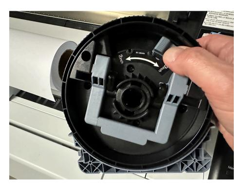
Release (lift) the adapter lock on both roll paper adapters.
