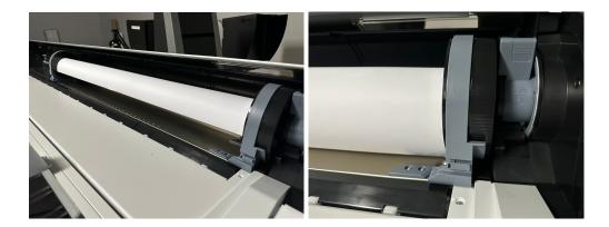
On the printer Control Panel press load/remove paper button.
