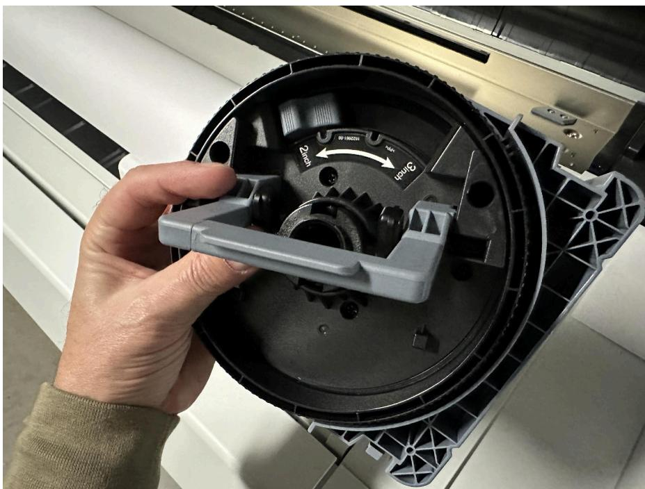
Push adapters into the paper core at both ends of the roll and push down the adapter lock levers flat against the adapters.
