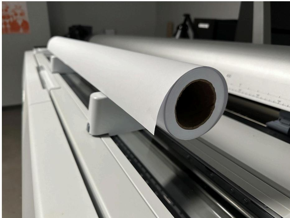
Lift the cover at the back of the printer and take out both roll paper adapters.
