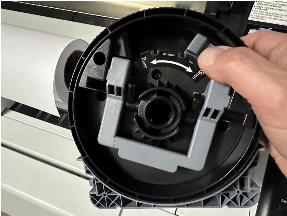
Release (lift) the adapter lock on both roll paper adapters.
